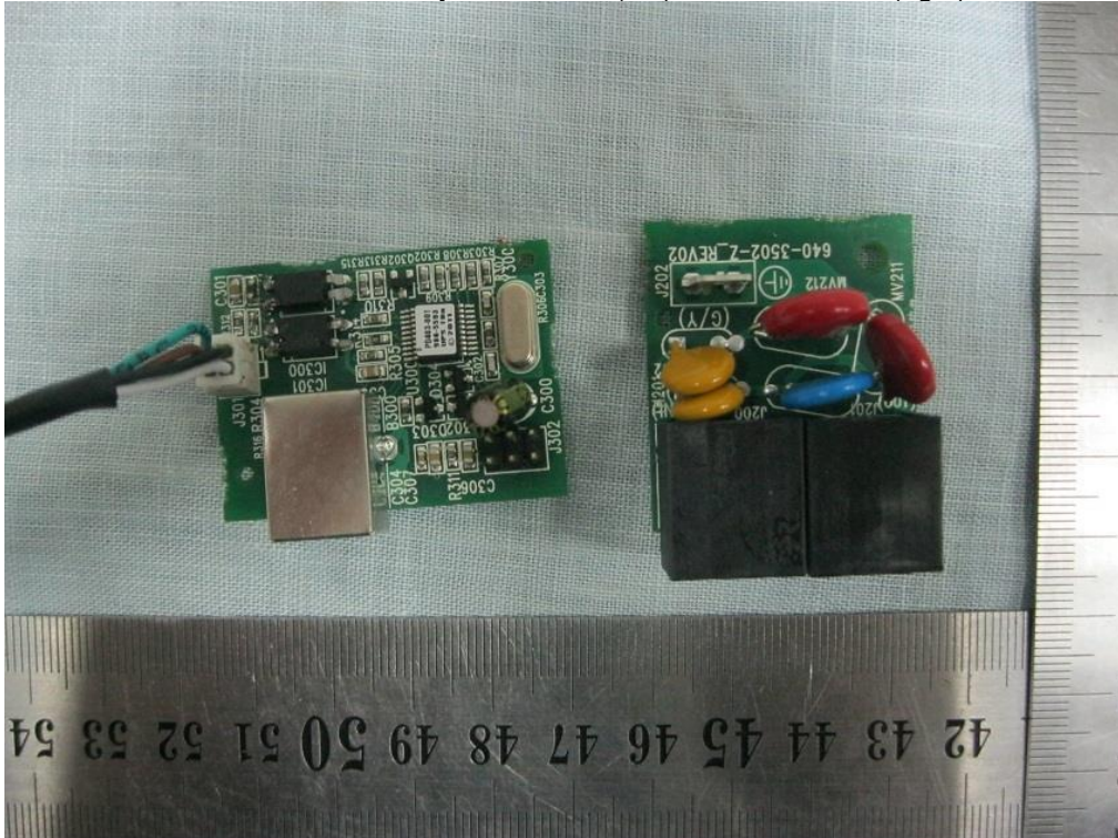
For model SX31K1CI; SX31K1CIy USB board (left) and TNV board (right)
